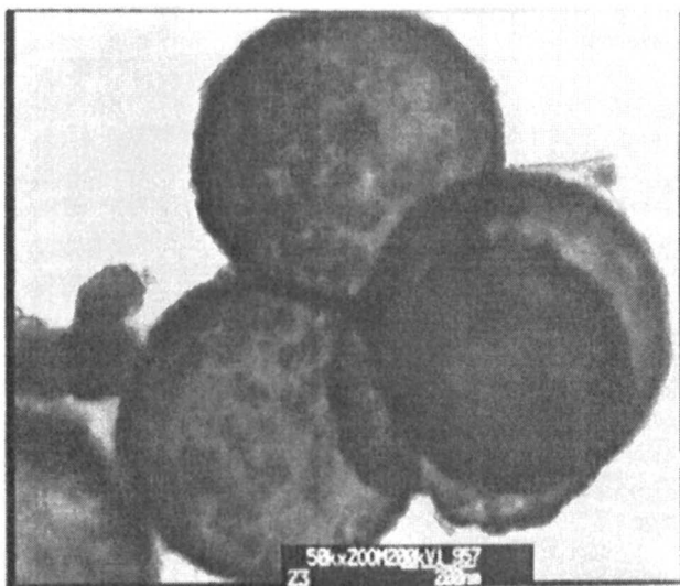
Figure 2. TEM image showing cross-section of PbS film coating 0.827 \mu\text{m} polystyrene core.
