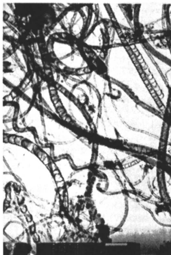
Figure 6. High-resolution transmission electron micrograph of polyethyleneimine-modified carbon nanotube (40,000 x)
